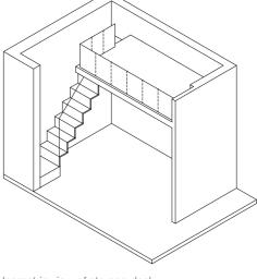
Isometric view of storage deck Clear ceiling hight of 3.2m
